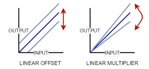
Since it takes two points to define a line, most linear calibrations will be performed using two points. Per the diagram below, note that points A and B will shift according to their applied offset or multiplier.
