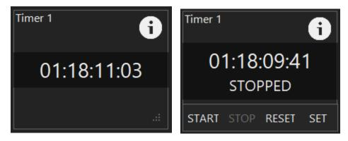
To create a Timer Element, select 'Menu... Add Timer'. Timers support User Control, and have specific properties to count up or down, which is selected in the 'Timer Type' property. The default value the timer becomes when it is reset is defined in the 'Reset Value' property.
