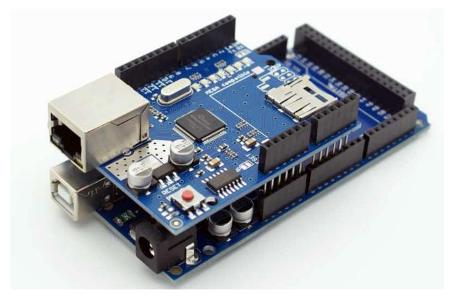
When plugging shields in, be careful that the pins are appropriately aligned and squeeze together along the headers, not the middle of the boards.
