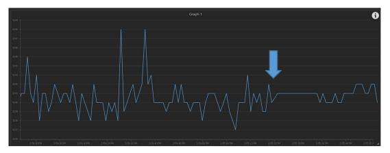
For example, here is a graph of a sensor where the 'Avg Weight' property was changed from 100% to 20% at the arrow:
