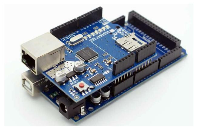
When plugging shields in, be careful that the pins are appropriately aligned and squeeze together along the headers, not the middle of the boards.
