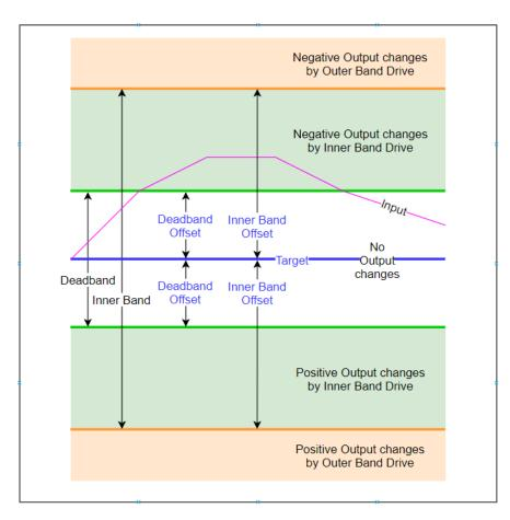
In the above graphic, an example input, such as a temperature in a heating control circuit. When the input is inside the Deadband, the output driving the control circuit remains constant. When the input enters the inner band, the output is reduced with each calculation cycle, and in this example, allows the input to follow suit.
