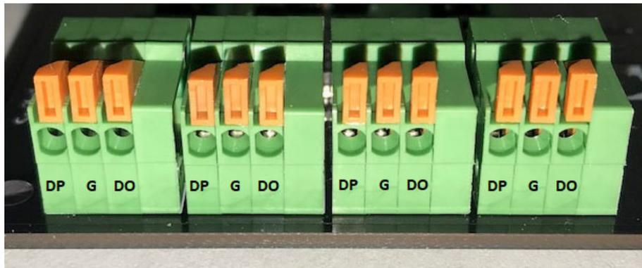
DP terminals connect directly to the associated Feather pin. These can be used for low-current outputs, inputs, 1-wire sensors, etc. just as if the wiring were being directly connected to the Feather. Where used as an output, the current limitations for that particular Feather must be followed (e.g. 10 mA @ 3.3 VDC max).
