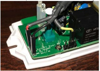
17. Retract the Temperature Probe wire through the main case body hole until there is just enough slack once the main case body is installed back on the bottom plate. Loop a nylon tie inside the case around the Temperature Probe wire and pull it tight to create a strain relief inside the case. Trim the tie's loose end. Alternatively, use a larger piece of heat-shrink tubing to create a larger diameter wire which cannot retract back out of the hole any further.
