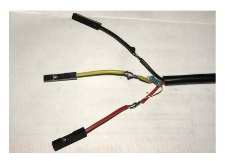
16. Plug the female connector with the black wire to the GND pin of the new header. Plug the female connector with the red wire to the VCC pin of the new header. Plug the female connector with the yellow wire to the BUTTON 1 of the existing header.
